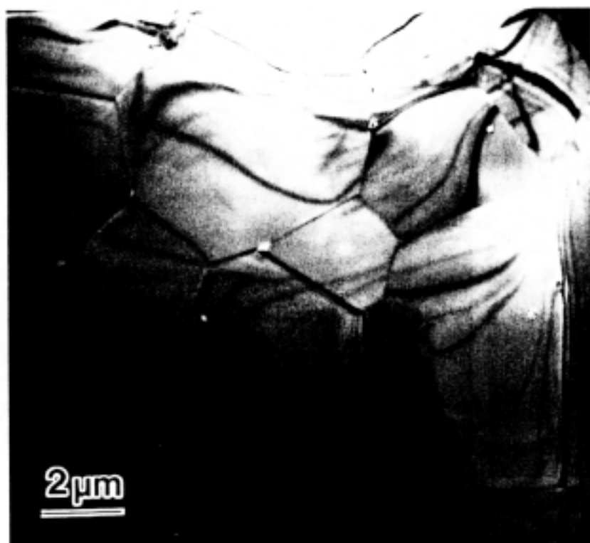
Fig. 5. TEM micrograph of sintered (1280 °C, 4 h) ZnO microstructure
