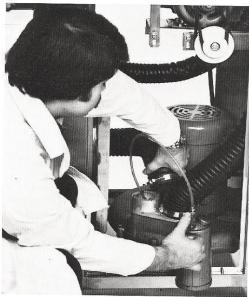
Removing intake hose and spraying paraffin oil
