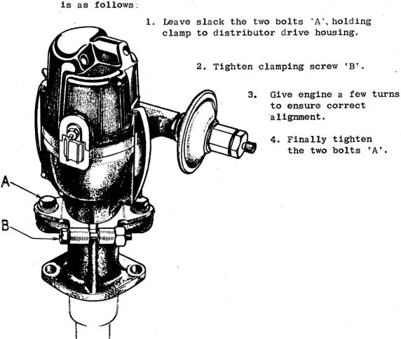
4. Finally tighten the two bolts 'A'.
