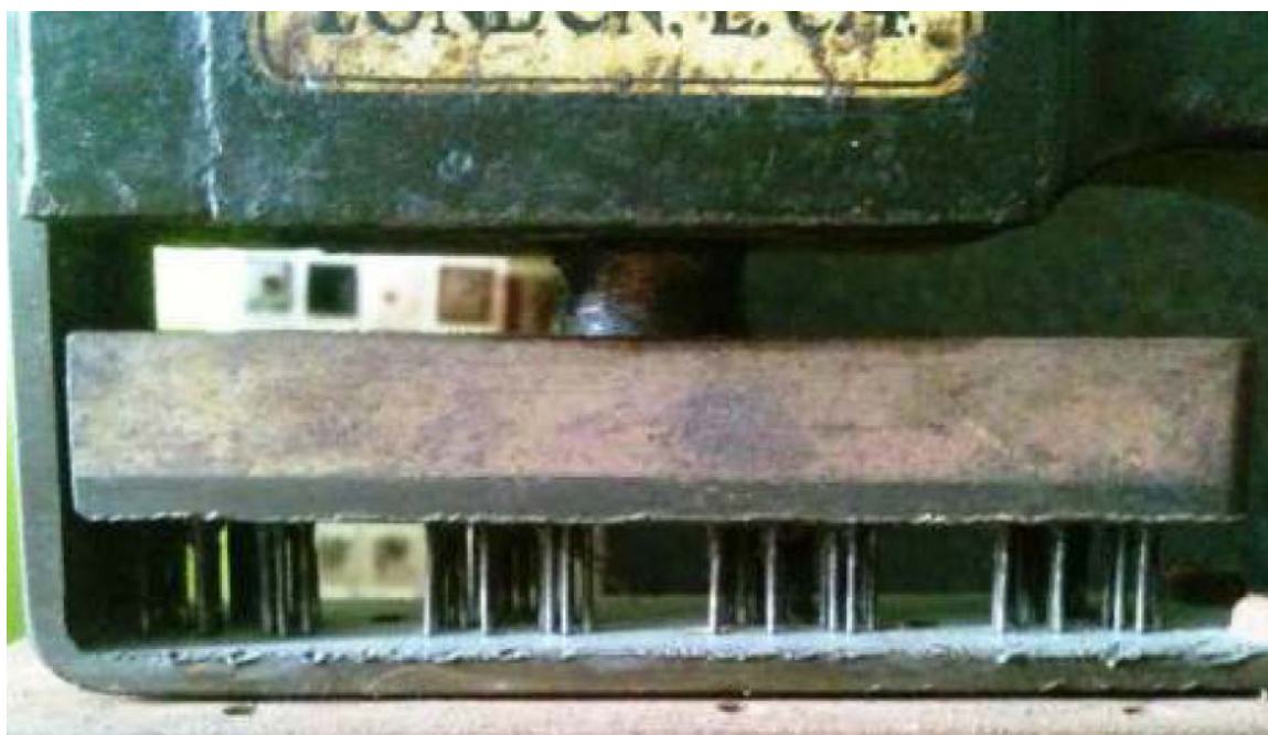
Fig. 3 – Close-up platen showing the pins.
