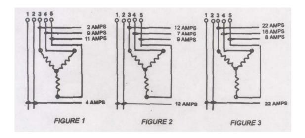
\*\*\*Note: Figure 1: On the single-phase power in on L I and L2 when a motor is running at no
