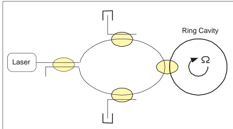
Figure 5.1: Resonator fiber-optic gyro (R-FOG) elementary configuration
