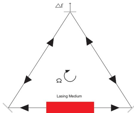
Figure 2.1: Ring Laser Cavity
