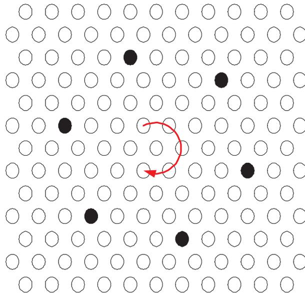
Figure 5.2: A ring resonator in a photonic crystal
