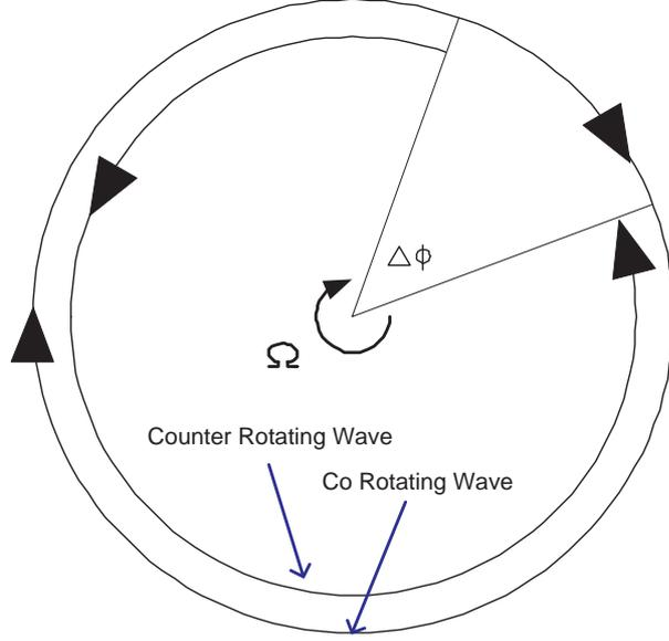
Figure 1.1: Phase shift between two counter-propagating waves
