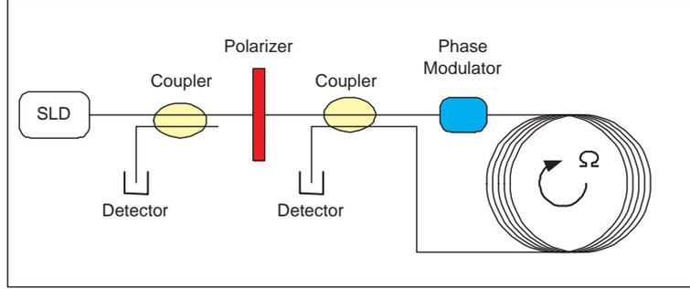
Figure 3.1: Elementary configuration of an I-FOG
