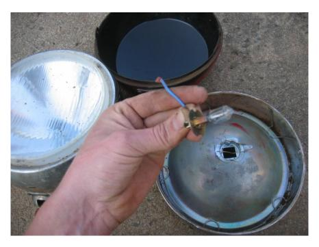
Undo the two side screws and remove the front housing. Remove the old Halogen bulb.
