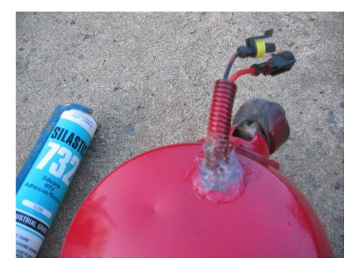
If a  $\frac{3}{4}$  inch hole was drilled, apply silicon sealant around the wires. Try and do a nicer job than I did.
