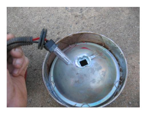
Insert the HID bulb taking care not to touch the bulb with your fingers. Make sure that the locking wire is in place to hold the bulb securely.
