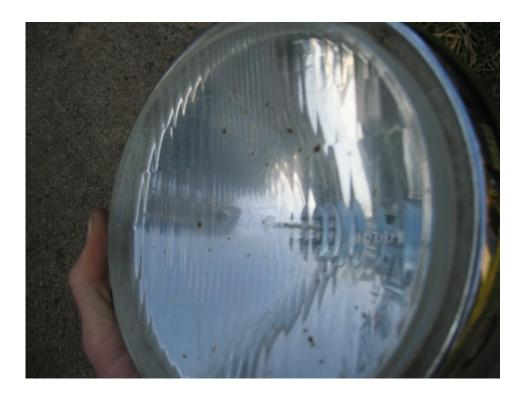
Slightly hard to see, but your HID bulb within the IPF 900 light should look something like this. The position of the arc in the H3 HID bulb is identical to that of the filament wire within a standard Halogen H3 bulb, thus giving the same optics but about 3 times brighter.
