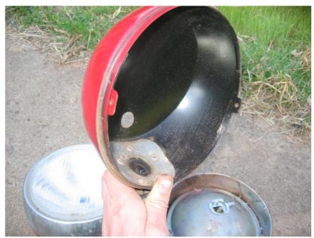
A ¾ inch hole is the smallest hole that is needed to allow the waterproof plugs to pass through. Silicon sealant will be required. If possible, drill a 22mm hole and the included rubber grommet can be utilised.
