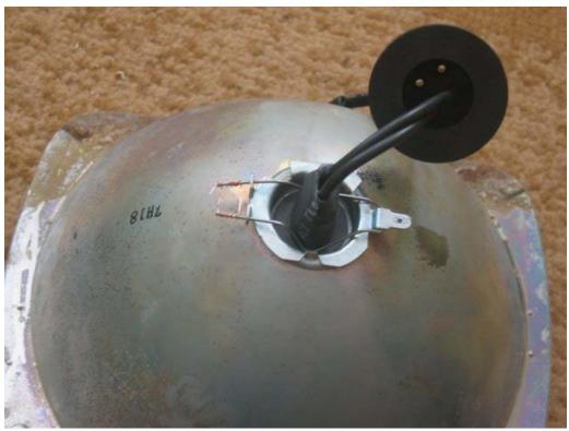
If your bulbs came with rubber grommets already installed on the leads, depending on the size drill the required size hole in the rear of the IPF housing. The above piccy will need a a ¾ inch hole. The waterproof plugs will pass through a ¾ inch hole fine. Apply silicon sealant around the wires and the grommet. Try and do a nicer job than I did. The position of the arc in the H3
