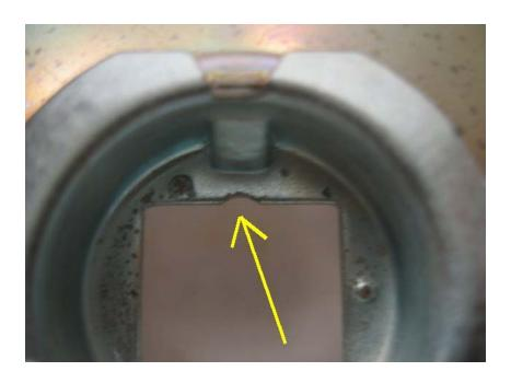
A notch may need to be filed depending on the type of HID bulb. Use a small file to do the job.
