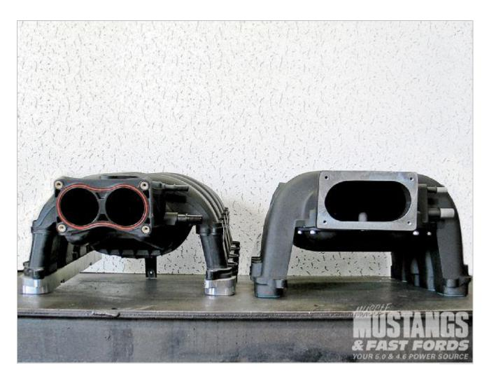
Next it was the C&L intake manifold's turn, and equipped with the GT500 throttle body, peak power improved to 429 hp. Bender told us that a single-blade throttle body wouldn't disappoint, and it didn't as it increased power output to 435.90. The C&L piece really flows some air, so the better throttle body is needed to make sure it lives up to its potential. While the single was worth some 7 hp at peak power, in other areas under the curve, it was good for as much as 8-9 rwhp.
