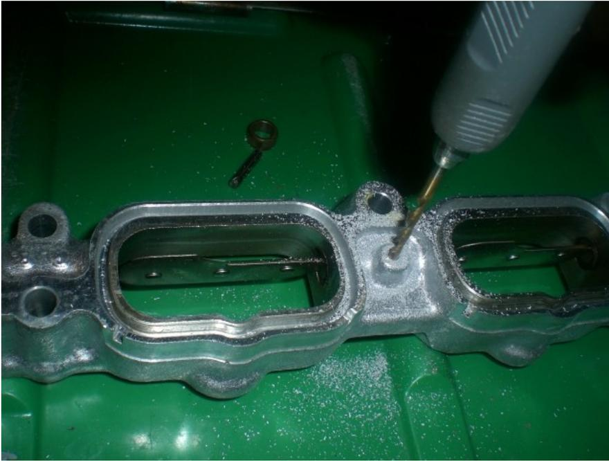
**After doing this u could use a nail or a piece of metal and the hammer to take the retainer pin as show**
