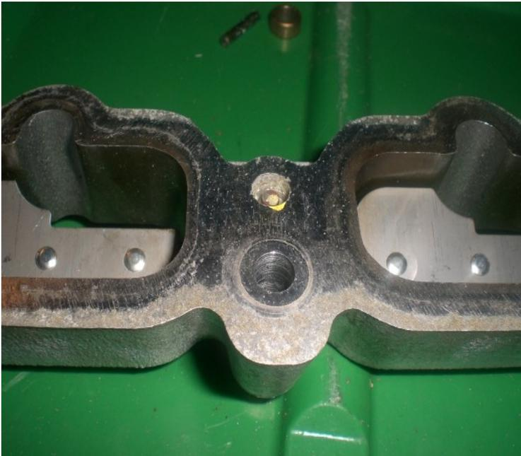
**To turn take it out just flip it over. Drill a hole right in the spot where the pin is until u can see the pin.**
