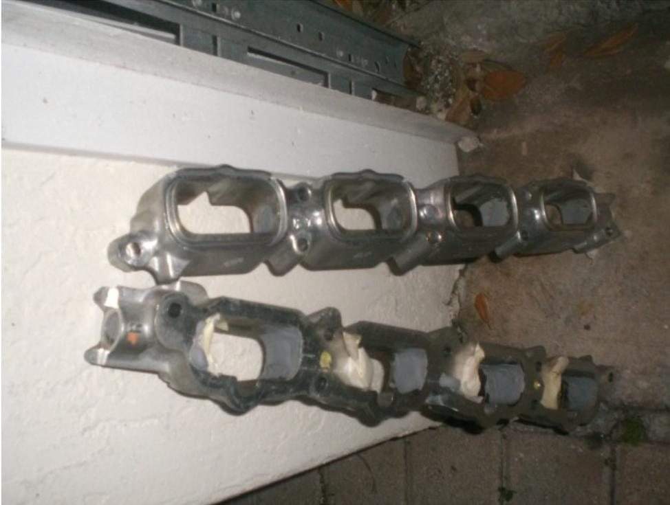
**Now let it dry and harden it takes a few minutes but I rather left it for 24 hours. After its hard enough I can start using the rotary tool with the stones, sanding polishing tips**
