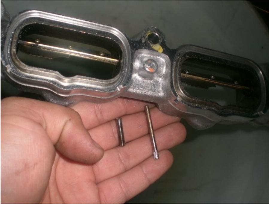
**With the pin out now you can go on and remove the butterflies off. To do this you could either use the drill or the rotary tool with a stone.**
