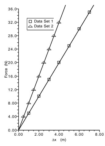
The graph at left was made from data collected during an investigation of the relationship between the amount two different springs stretched, when different forces were applied.
