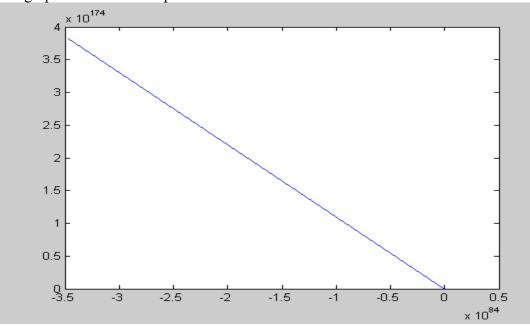
With RK4  $\mu$ = 500 it does not converge for any reasonable values of N. This graph is the failed output from the RK4.
