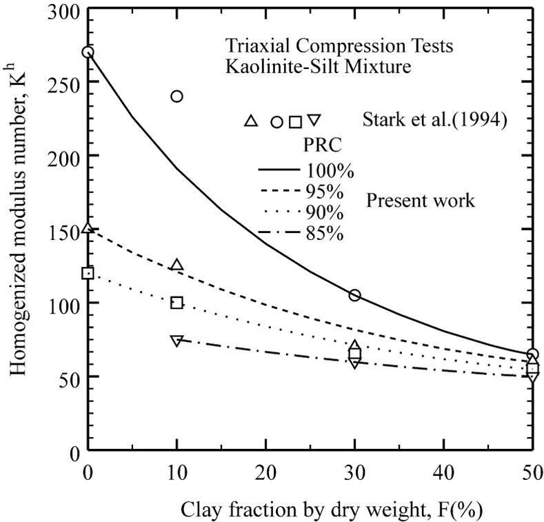
Fig. 5. Young's modulus number at different Proctor relative compaction (PRC).
