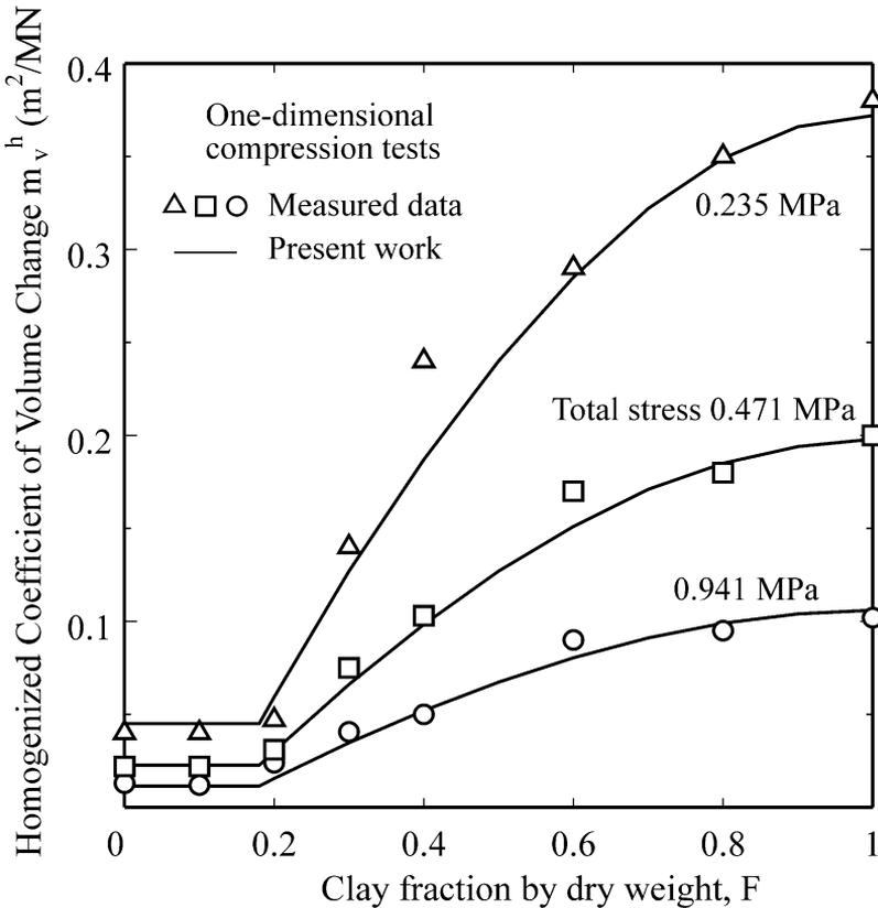
Fig. 8. Homogenized coefficient of volume change for mixed soil A.
