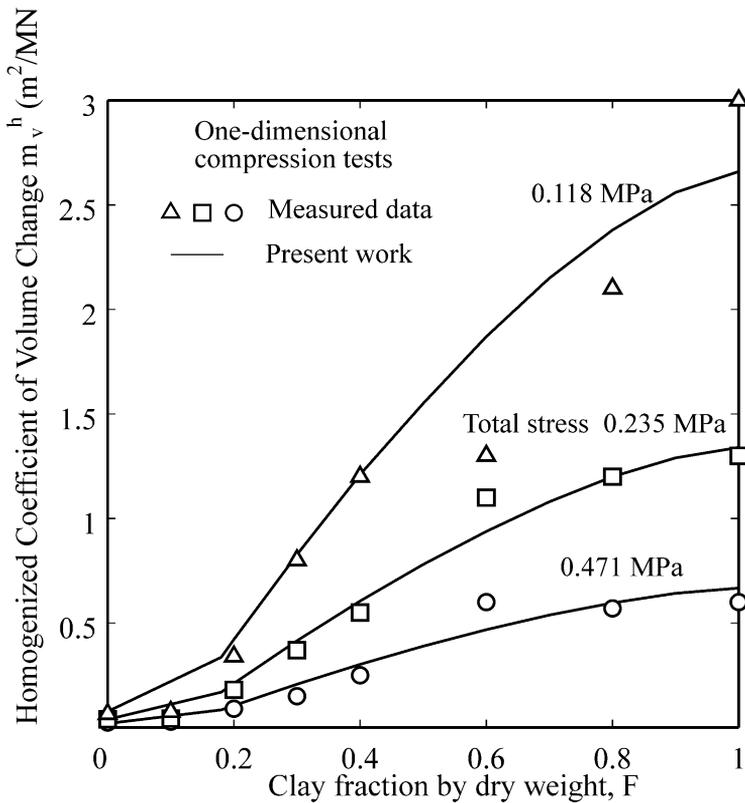
Fig. 9. Homogenized coefficient of volume change for mixed soil B.
