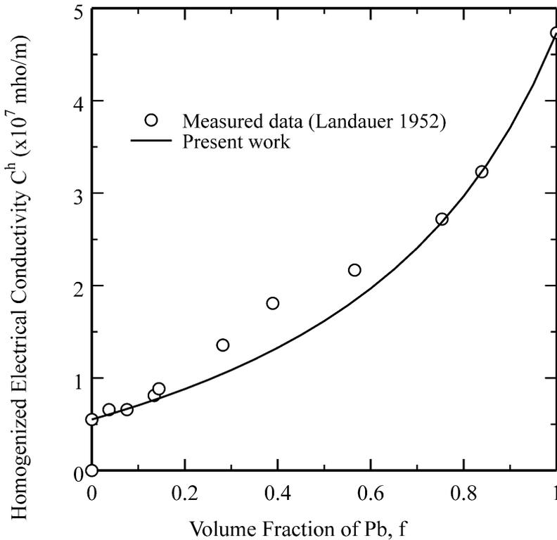
Fig. 4. Comparison of theoretical prediction and experimental data for electrical conductivity of  $Mg_2Pb - Pb$  mixture.
