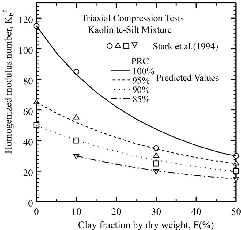
Fig. 6. Bulk modulus number at different Proctor relative compaction (PRC).
