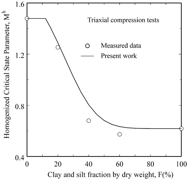
Fig. 11. Critical state parameter for mixed soil B.
