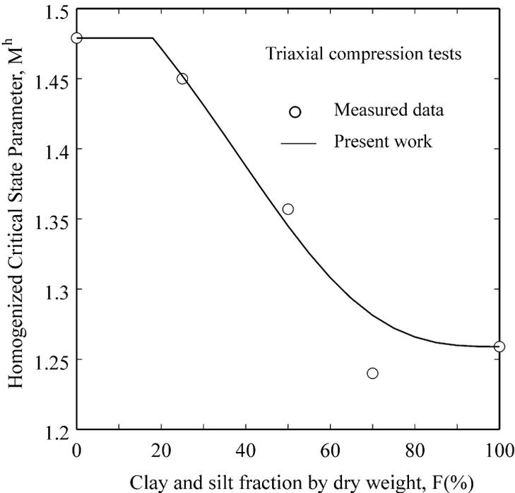
Fig. 10. Critical state parameter for mixed soil A.
