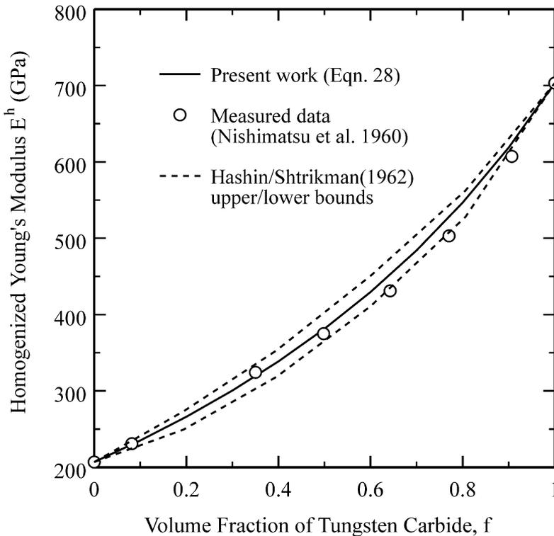
Fig. 3. Comparison of homogenized Young's modulus of a two-phase alloy.
