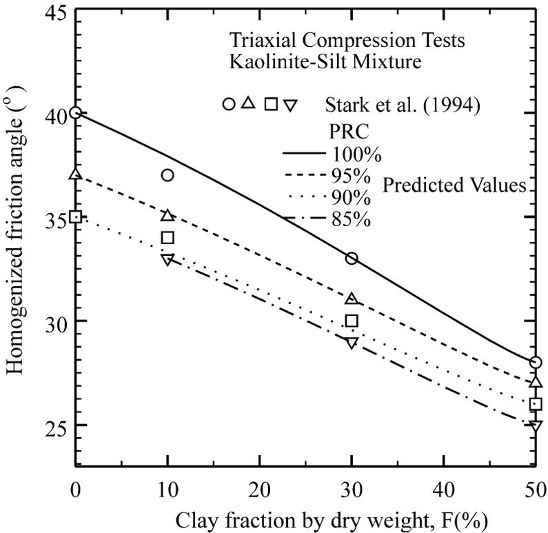
Fig. 7. Friction angle at different Proctor relative compaction.
