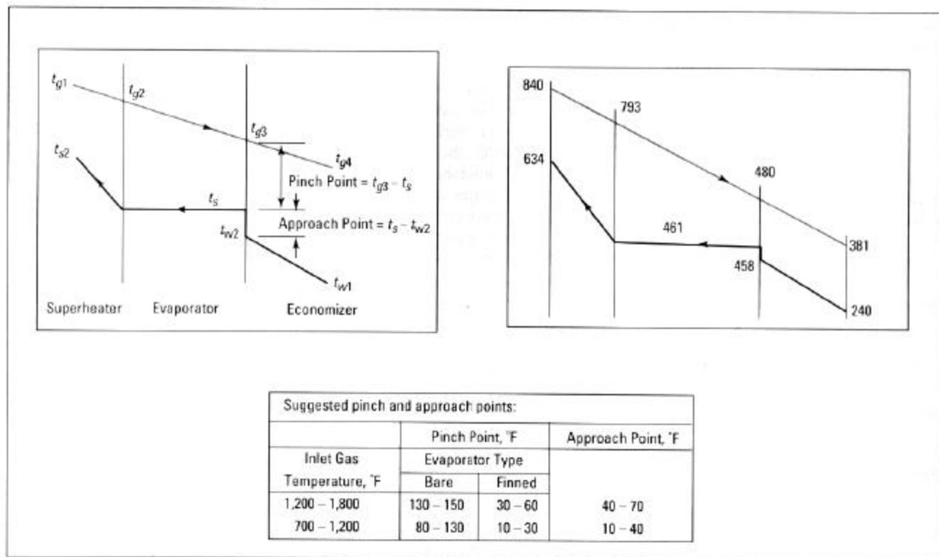
■ Figure 2. HRSG temperature profiles and suggested pinch and approach points.
