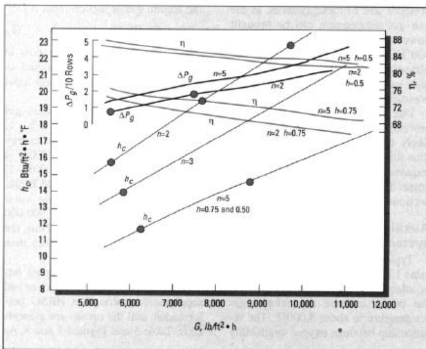
■ Figure 6. Effects of fin configuration on heat transfer and pressure drop.
