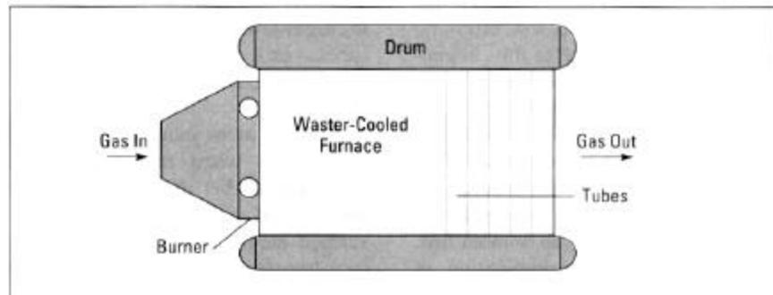
■ Figure 5. Exhaust-fired HRSG.
