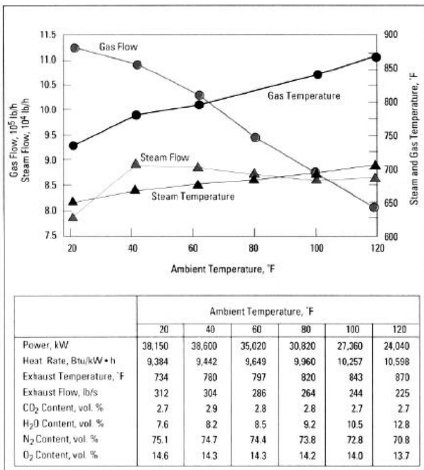
■ Figure 12. Effect of ambient temperature on HRSG performance.
