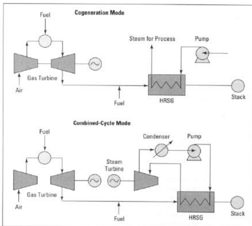
■ Figure 1. HRSGs can be operated in either the cogeneration mode (top) or the combined-cycle mode (bottom).
