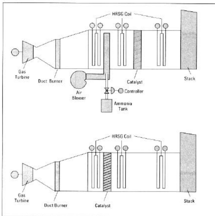
■ Figure 11. Catalyst arrangements for  $\text{NO}_x$  and CO reduction.
