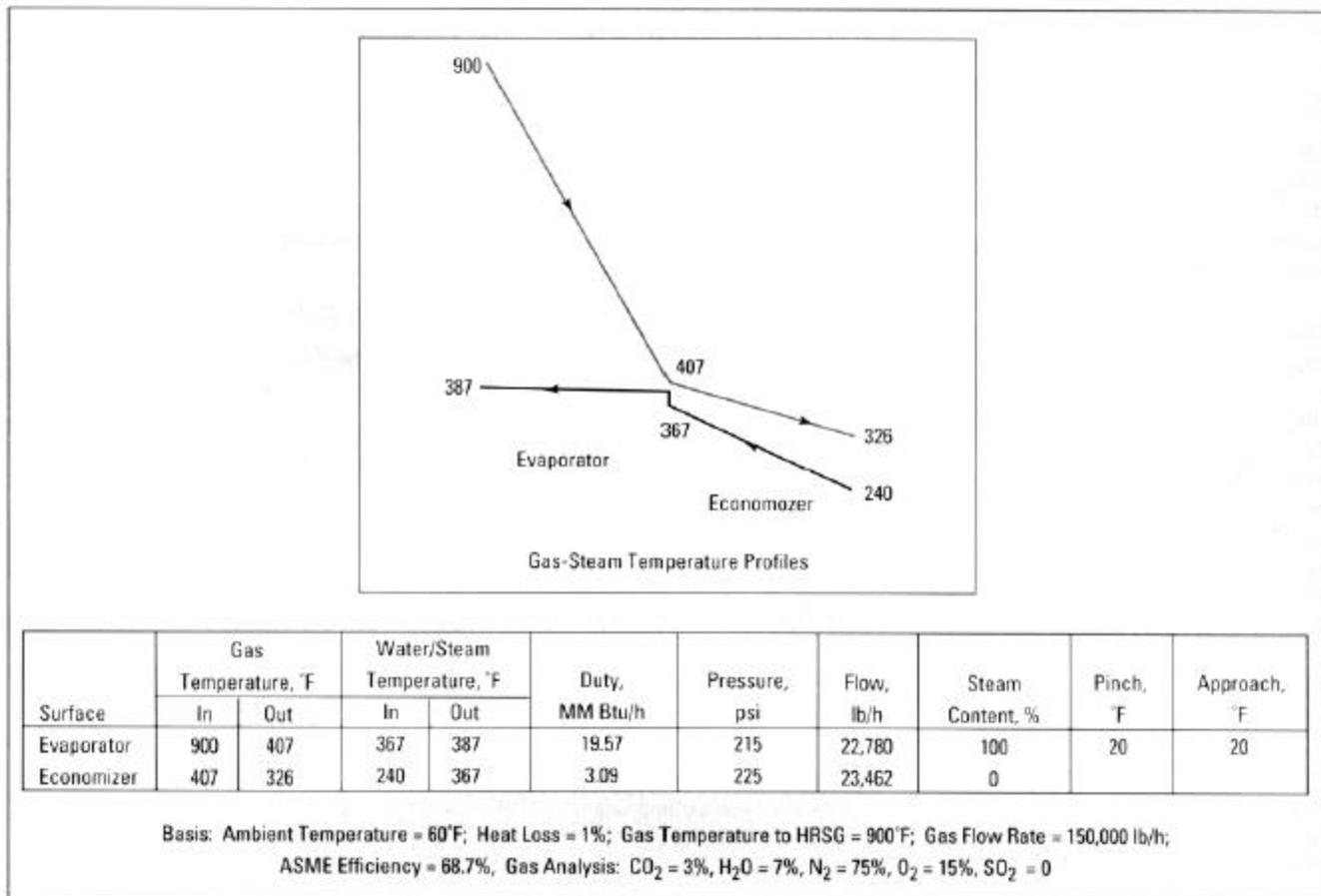
■ Figure 7. Simulated performance of HRSG without supplementary firing.
