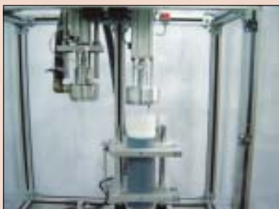
7. A pneumatically controlled cylinder inserts the plunger.
