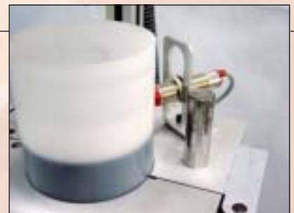
6. A sensor keeps the filling level constant. Optional: digital weighing scale.
