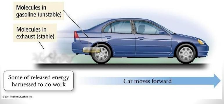
The car engine is a special mechanism that transforms the **usable** chemical energy in the gasoline into the work of the car moving forward.
