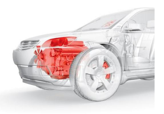
The car engine is **heat engine** because it first transforms the chemical energy of the gasoline molecules into heat by burning the gasoline with oxygen from the air (Heat of reaction).
