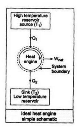
The first law tells us that the quantity of high-temperature heat (thermal energy) that is consumed is equal to the sum of the quantity of work produced plus that of the discarded low-temperature heat: the total amount of energy is conserved.
