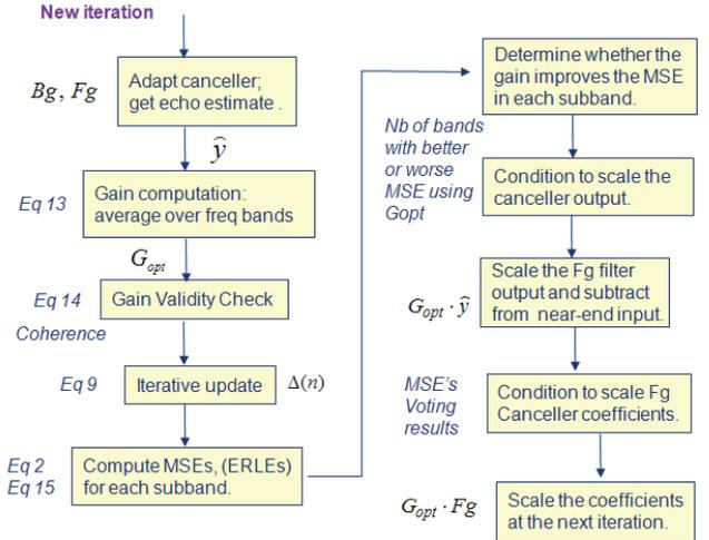
Figure 5. Algorithm Flowchart
