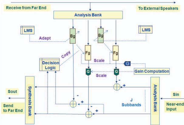
Figure 4. Subband-based 2-path Architecture
