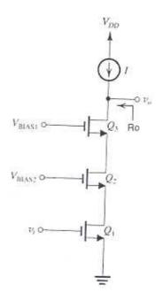
(5 pts) If all transistors in the above circuit have identical  $r_o$  and  $g_m$ , what is the output resistance Ro at the output of this circuit?
