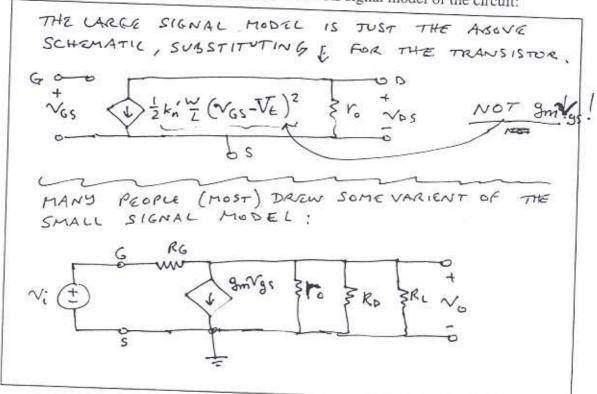
Let the following NMOS transistor have a V<sub>t</sub> of 1V,  $\mu_{\rm B}C_{\rm ox}$ =200  $\mu$ A/V<sup>2</sup>,  $\lambda$ =0, L=1 $\mu$ m, and W=10 $\mu$ m. Set V<sub>dd</sub>=10V.
