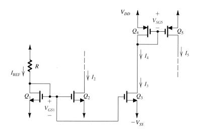
In the above schematic,  $I_{REF}=1$  mA,  $I_2=0.5$  mA,  $I_3=I_4=4$  mA, W/L of  $Q_1=3/6$ , W/L of  $Q_2=2/X$ , W/L of  $Q_3=Y/3$ , W/L of  $Q_4=100/2$ , and W/L of  $Q_5=2/100$ . Showing your work, find X, Y, and  $I_5$ .
