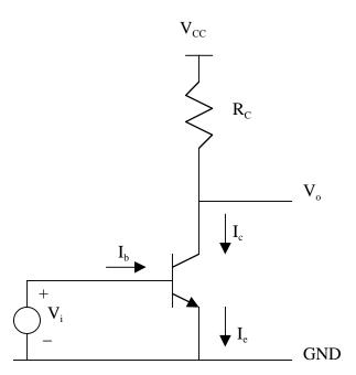
(6 pts) Draw and completely annotate a **large** signal equivalent circuit model for this amplifier. Do not draw the small signal model here!
