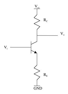
(5 pts) Draw the small signal equivalent circuit model for this amplifier:
