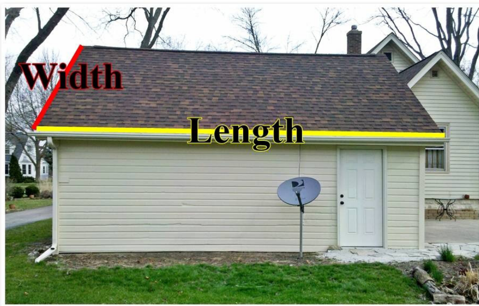
Figure 4: Determining the surface area of the roof.
