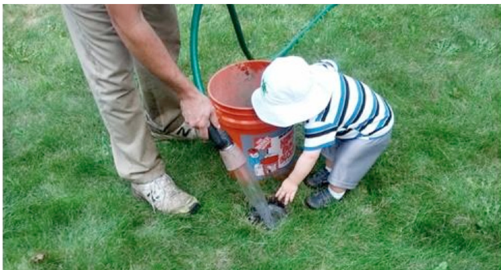
Figure 11: Fill up the test hole with water.
