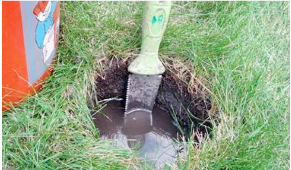
Figure 12: In summertime, the test hole may drain quickly, the installer or homeowner must refill every 15 minutes for 1 hour to accommodate for different seasonal soil moisture conditions.
