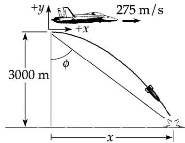
(b) The plane has the same velocity as the bomb in the  $x$  direction.
