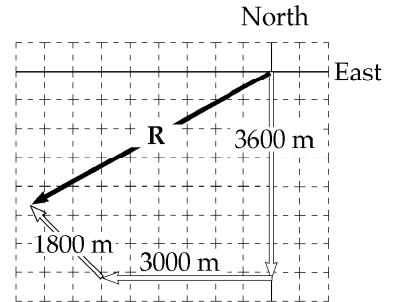
(a) Net displacement =  $\sqrt{x^2 + y^2} = \boxed{4.87 \text{ km at } 28.6^\circ \text{ S of W}}$
