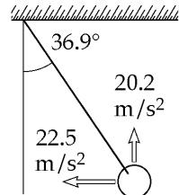
(c)  $a_c = \frac{v^2}{r}$  so  $v = \sqrt{a_c r} = \sqrt{29.7 \text{ m/s}^2 (1.50 \text{ m})} = 6.67 \text{ m/s}$  tangent to circle
