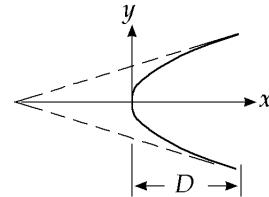
Thus the horizontal distance from the aperture to the virtual source is  $2D$ . The source is at coordinate  $x = -D$ .
