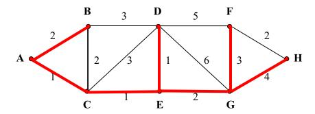
(ii) The minimum spanning tree joining the nodes:
