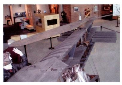
The front of the fuselage had the circular locating cuff for the engine cowl cut off, and the opening was covered over with plastic sheet. A hole was drilled in the middle to take the engine.
