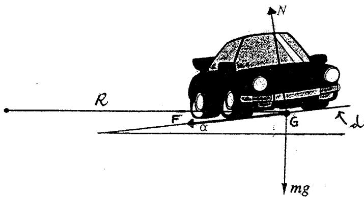
A car of mass  $m$ , represented by the point  $G$ , is travelling at constant speed  $v$  around a curve of radius  $R$  on a road of width  $d$ . The road slopes at an angle  $\alpha$  towards the centre of the curve. The forces acting on the car are the gravitational force  $mg$ , a sideways friction force  $F$  (acting down the road as drawn) and a normal reaction  $N$ , at right angles to the road.
