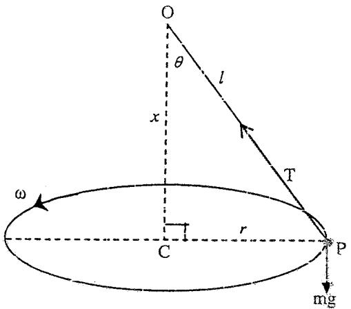
A conical pendulum consists of a bob  $P$  of mass  $m$  kg on the end of a string  $l$  metres long. The bob rotates in a horizontal circle of radius  $r$  and centre  $O$  at a constant angular velocity  $\omega$  radians per second. The angle that the string makes with the vertical is  $\theta$  and  $CO = x$  metres. The forces acting on the bob are a gravitational force of  $mg$  newtons and a tension in the string of  $T$  newtons.
