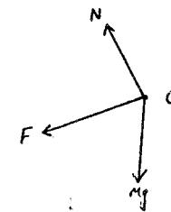
Forces on the car are gravitational force  $Mg$  down, normal reaction force  $N$  and friction force  $F$ .Resolving vertically
