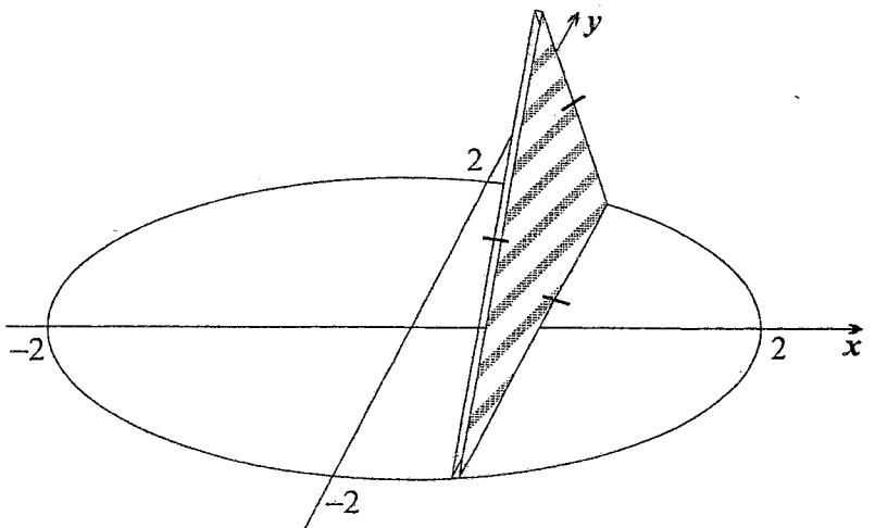
The diagram above shows a cross-sectional slice of a solid whose base is the region enclosed by the circle  $x^2 + y^2 = 4$ . Each such cross-section of the solid is an equilateral triangle. Find the volume of the solid. 4
