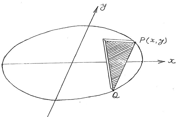
The base of a particular solid is an ellipse with major and minor axes of 10 cm and 8 cm respectively. Every cross-section perpendicular to the major axis is an equilateral triangle one side of which lies in the base of the solid as shown above.
