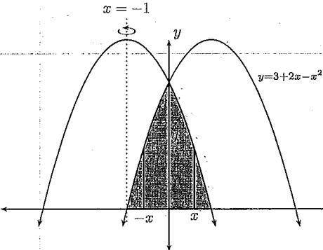
The diagram above shows the parabola  $y = 3 + 2x - x^2$  and its reflection in the  $y$ -axis. The vertical strips shown will generate cylindrical shells of the same height  $y$  when rotated about the line  $x = -1$ .
