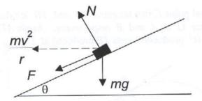
Given the radius of the curve is 1km and  $\tan \theta = \frac{1}{100}$  find the velocity in m/s which will ensure no sideways friction (i.e. F = 0). Take  $g = 10m/s^2$
