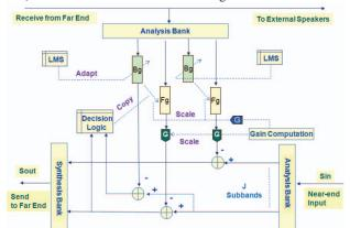
Figure 4. Subband-based 2-path Architecture
