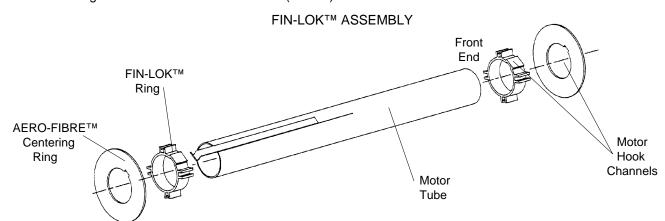
**NOTE:** FROM THIS POINT ON, DO NOT USE ANY CEMENT UNTIL REACHING ASSEMBLY STEP 5.
