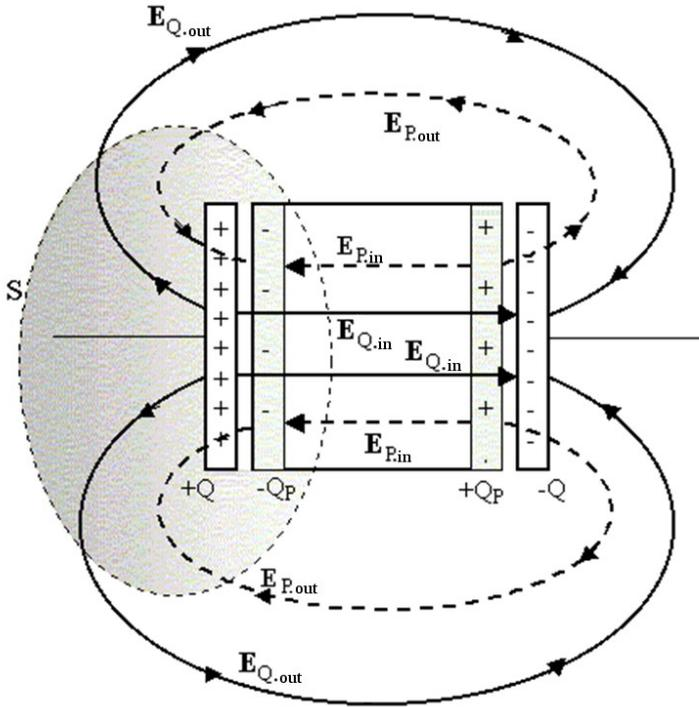
Fig. 2 – Pictorial representation of components of the electric field vector  $\vec{E}$  for a finite plate condenser with dielectric medium. P in index denotes the component which originates from resultant polarization charge  $Q_p$ , while Q in index denotes the component which originates from free charge  $Q$  on plates. (.in) in index relates to corresponding components inside the condenser, while (.out) relates to components outside the condenser.
