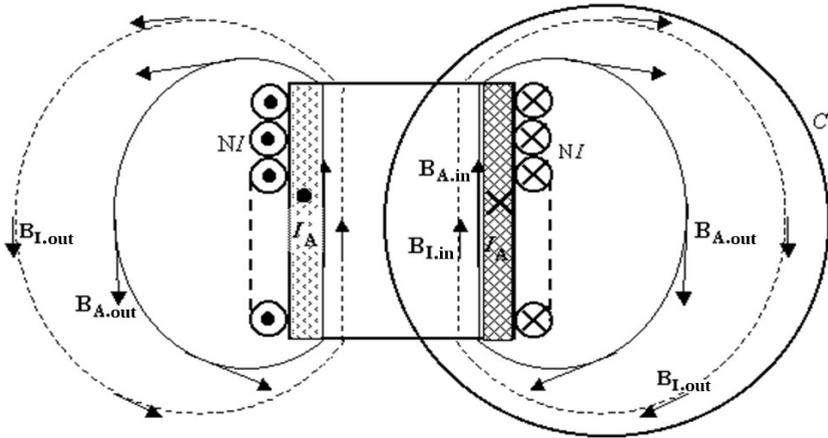
Fig. 1 – Pictorial representation of components of the magnetic field vector  $\mathbf{B}$  for a short solenoid with ferromagnetic core. “A” in index denotes the component which originates from resultant Amperian current  $I_A$ , while “I” in index denotes the component which originates from macroscopic currents  $NI$ . “in” in index relates to corresponding components inside the core, while “out” relates to components outside the core.
