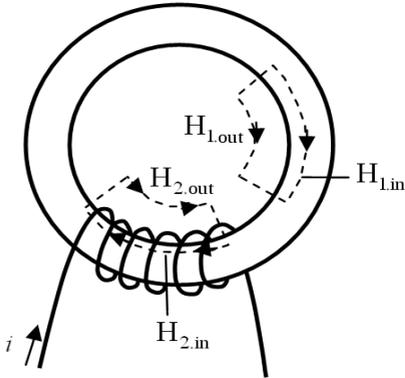
Fig. 4. Vectors  $\mathbf{H}_{1, \text{out}}$  and  $\mathbf{H}_{2, \text{out}}$  along concentric circles outside magnetic core have opposite directions.
