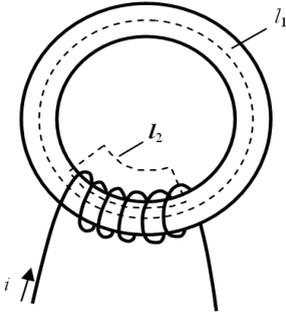
Fig. 3. An illustration of computation of vector field  $\mathbf{H}$ , where one gets two quite different values depending on path of integration.
