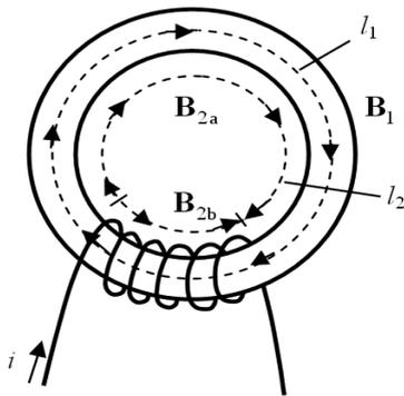
Fig. 5. One of the consequences of the "magnetic circuit theory" is the "sourceness" of the magnetic field vector, i.e. that a mere coil creates a pair of magnetic monopoles.
