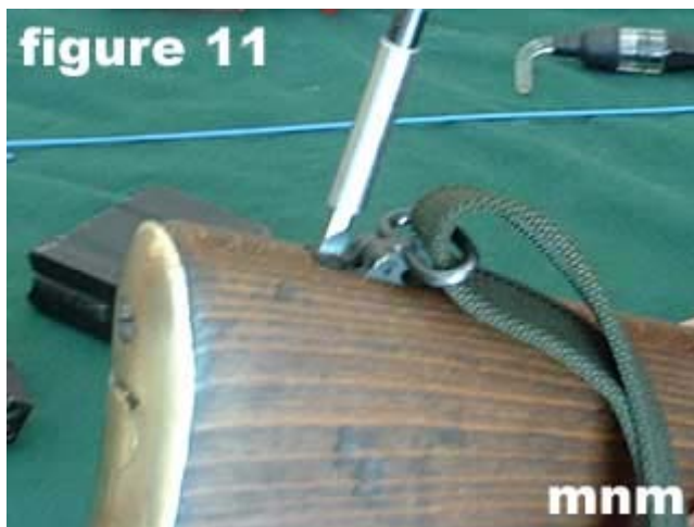
11) Unscrew both rear swivel screws .
