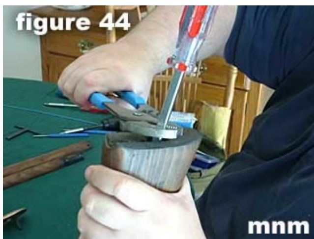
44) Using a pair of pliers, turn large flat blade screw driver clockwise until stock bolt is tight.
