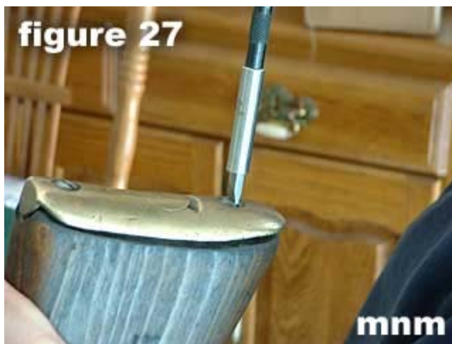
27) Loosen and remove buttplate screws .
