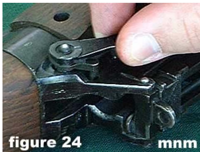
24) Remove the locking bolt and safety catch . Set aside assembled.
