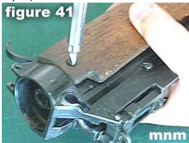
41) Tighten fore-end screw .
