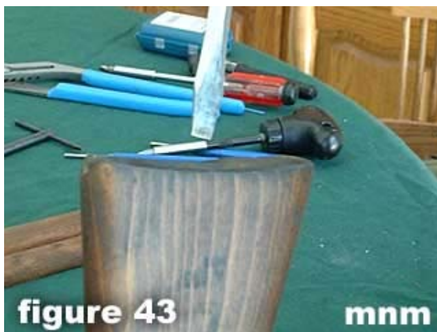
43) Insert a large flat blade screw driver into the butt stock trap .
