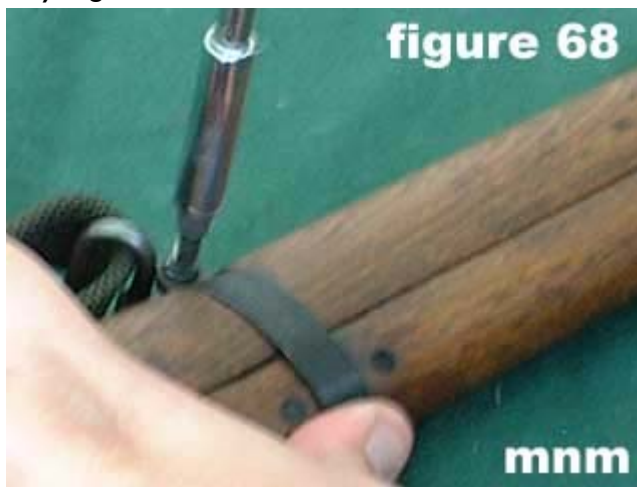
68) Replace and tighten the swivel band screw.
