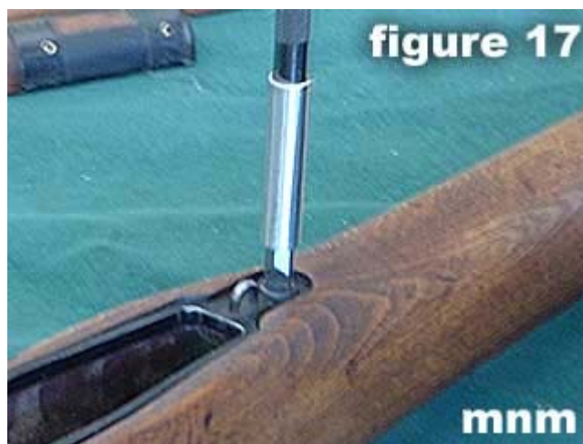
17) Unscrew front guard screw .
