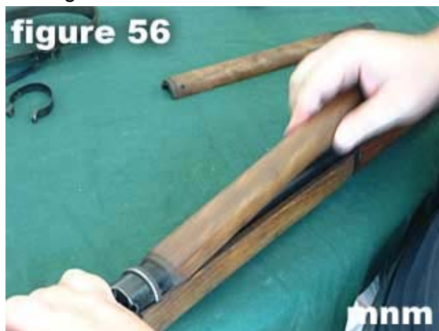
56) Reinstall rear hand guard.
