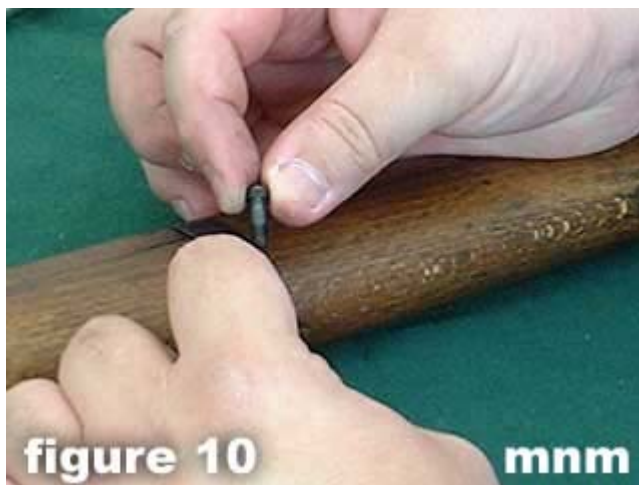
10) Remove the swivel band screw .
