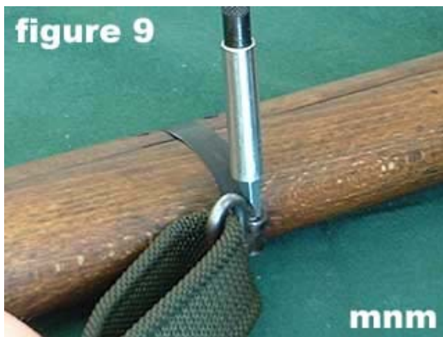
9) Unscrew the swivel band screw .
