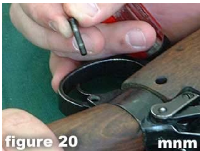
20) Remove rear guard screw.
