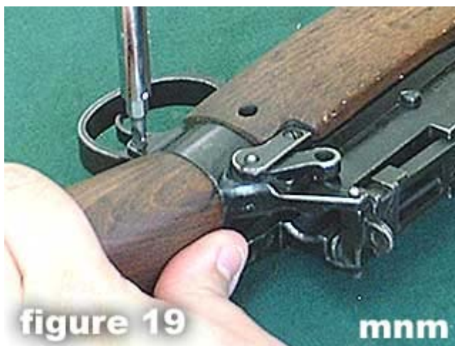
19) Unscrew rear guard screw.
