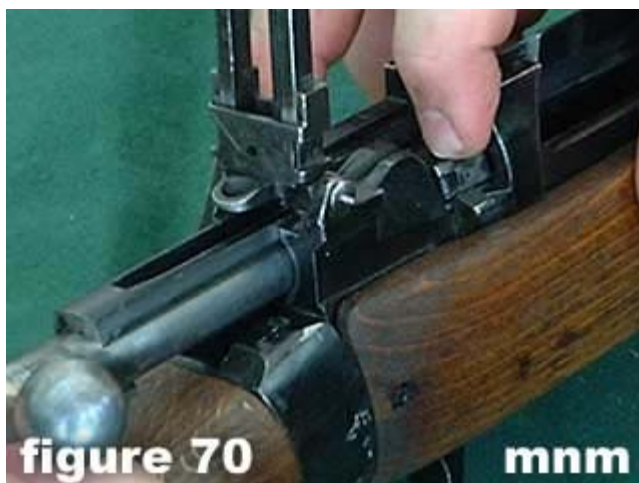
70) Insert bolt with breechbolt head point up. Depress bolt catch ( if rifle has one ).
