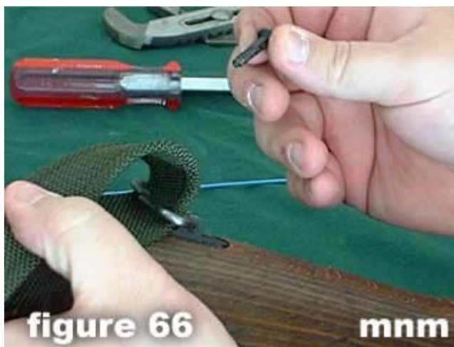
66) Reinstall the sling swivel.
