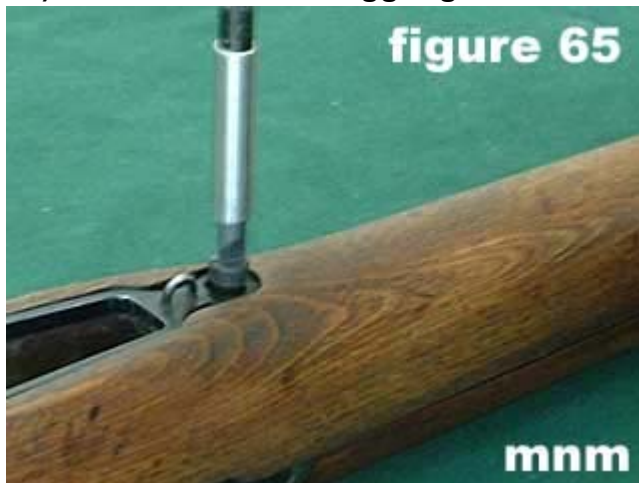
65) Tighten the front trigger guard screw.
