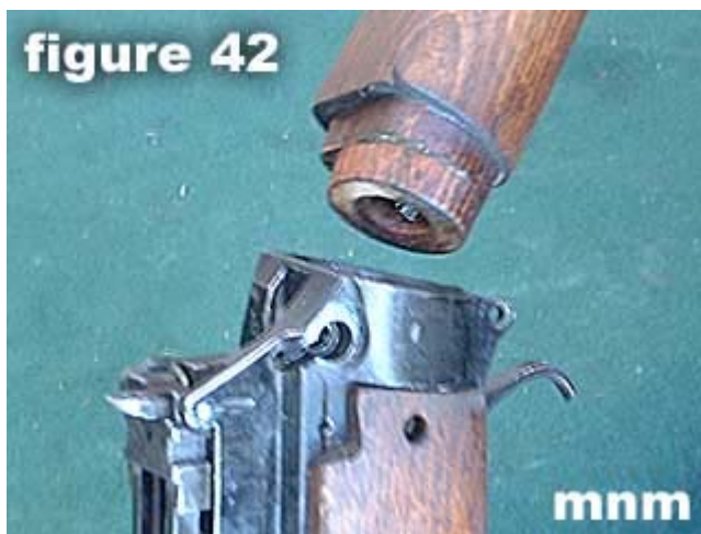
42) Reinsert buttstock into butt socket .
