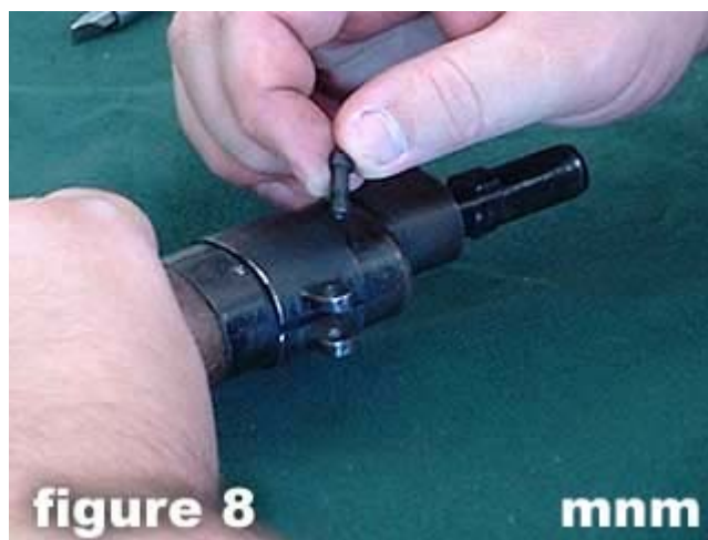
8) Remove the upper band screw .
