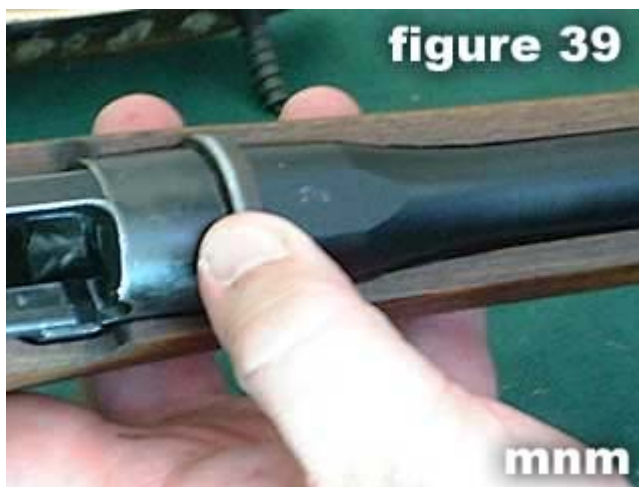
39) Make sure lower band is positioned correctly (as shown in figure 39 ).
