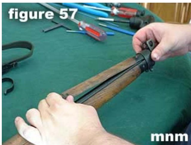
57) Reinstall front handguard . Make sure you install front under upper band and then pivot backwards.
