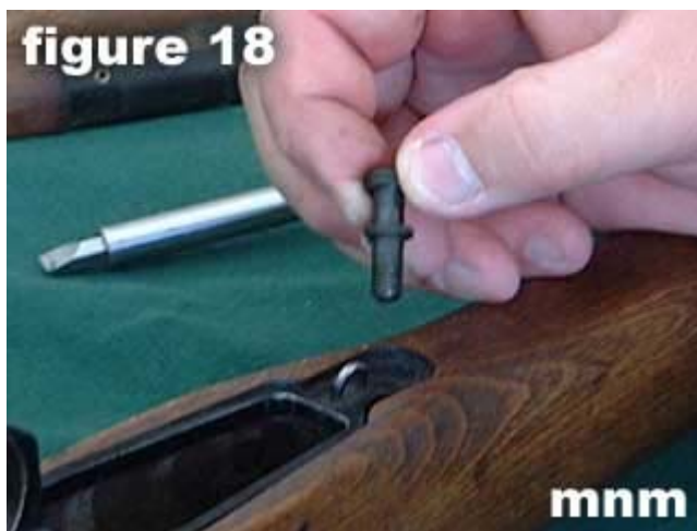
18) Remove front guard screw.
