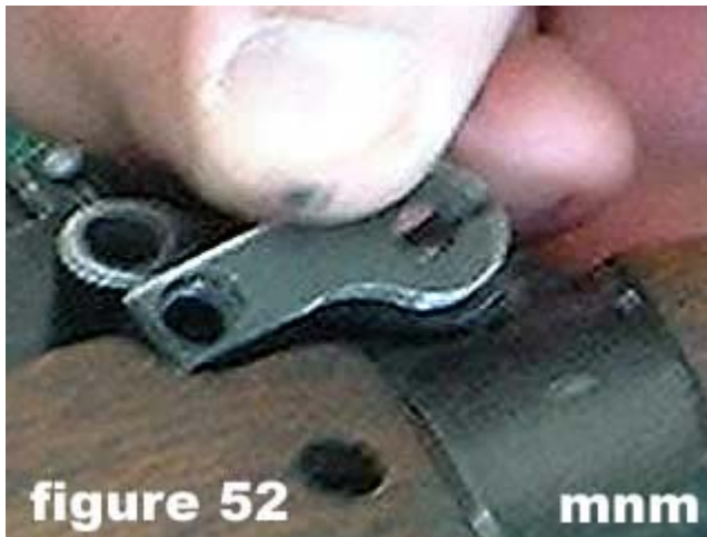
52) Figure 52 shows the safety spring . Note at the top of each part; the safety catch has a channel that the corresponding guide on the safety spring fits into to.
