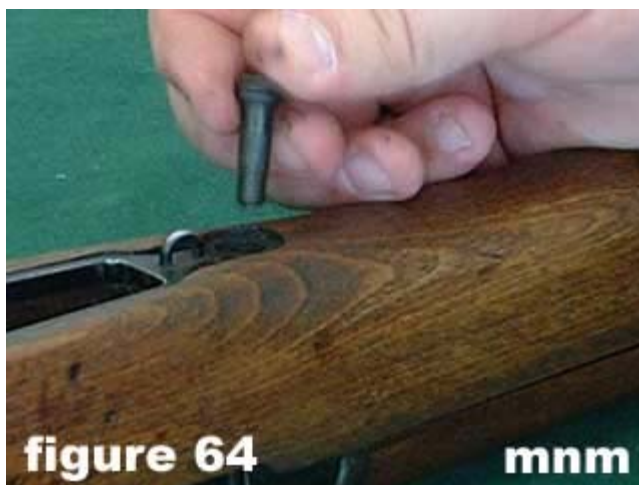
64) Reinstall the front trigger guard screw.
