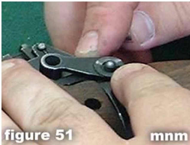
51) Install safety catch and locking bolt (as shown in figure 51 ).
