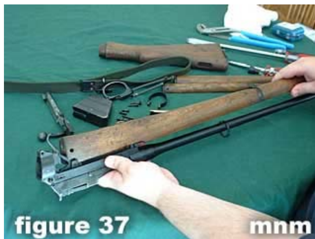
37) Pivot the fore-end stock into the butt socket (as shown in figure 37).
