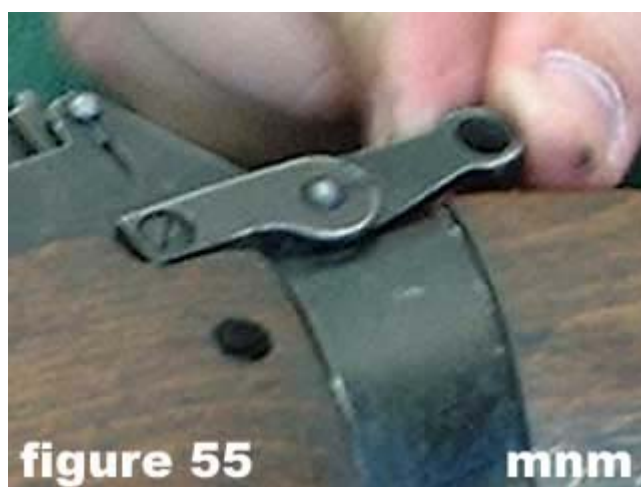
55) Make sure safety cycles on and off without binding.
