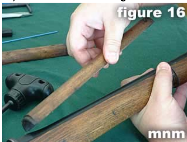
16) Remove the rear hand guard .
