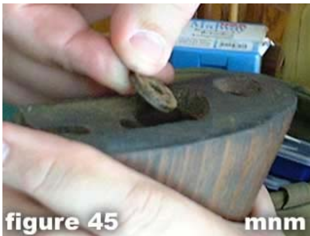
45) Reinsert the stock bolt wad into the butt stock trap of the butt stock.
