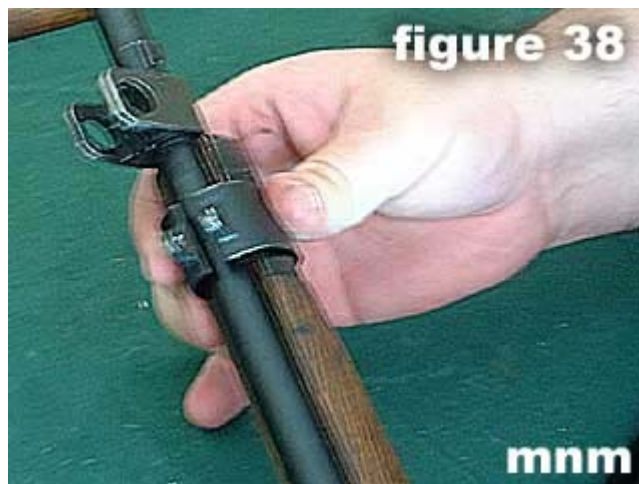
38) Reinstall upper band on barrel.
