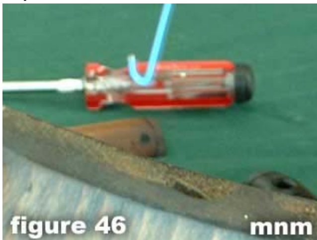
46) Using clothes hanger, push the stock bolt wad all of the way down until it rest flat on the stock bolt.
