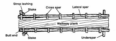
Each of the cross spars is lashed to the lateral spars with a square lashing, making three wraps and two fraps. (Refer to the "Lashing" section, page 63.) You can use any one of the three variations of square lashings mentioned in this pamphlet for the cross spars. The Japanese Mark II is the easiest and quickest to tie.
