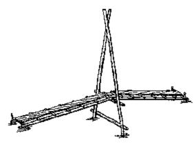
When the A frame is upright and the transom is level, lash both underspars on the walkways to the transom with strop lashings at three points. Finally, lash the cross spars at the ends of the walkways to stakes on the banks of the creek with strop lashings.
