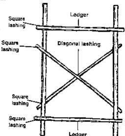
Diagonal lashing. After the ends of the ledgers and the cross braces are lashed to the legs, stand the trestle up on end. Adjust the trestle so that the legs are parallel. Also check to see that the top ledger is parallel to the ground. If it's not, lower the trestle, until the lashing, and adjust it.
