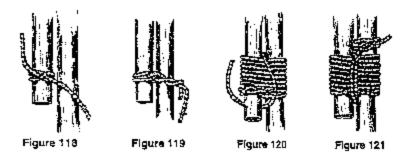
The two-spar shear lashing starts with a clove hitch on one spar (see figure 118). After making the clove hitch, wrap the excess part of the short running end around the standing part of the rope (see figure 119).
