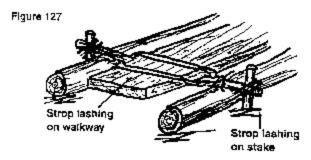
transom spar on the trestle) are lashed together at three points using a strop lashing (see figure 127).
