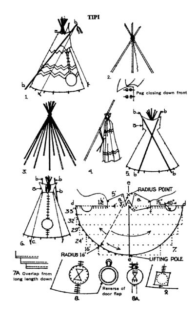
The tipi is entered through an opening which is closed with a piece of hide stretched over a light round frame of wood, much in the shape of a shield. This opening was usually decorated with the symbols of the owner. The opening could also be closed with just a hide or blanket hanging over it.
