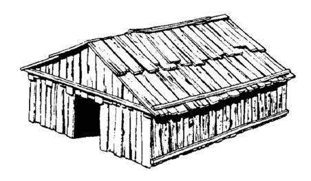
A plank house built entirely without nails. The parts were grooved and fitted together to support one another.
