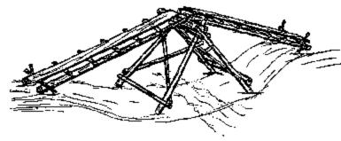
Next, the two walkways are put into position (see figure 133). Lash the underspars on the walkways to the transom spar with strop lashings at three points. Finally, the cross spars at the ends of the walkways are lashed to the stakes.
