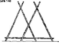
Double A frame. When you have four A frames, you can lash two of them together to form a double A frame (see figure 140). Lay one A frame on the ground and then put another on top so that the bottom ledgers overlap one-half their length (approximately 3').
