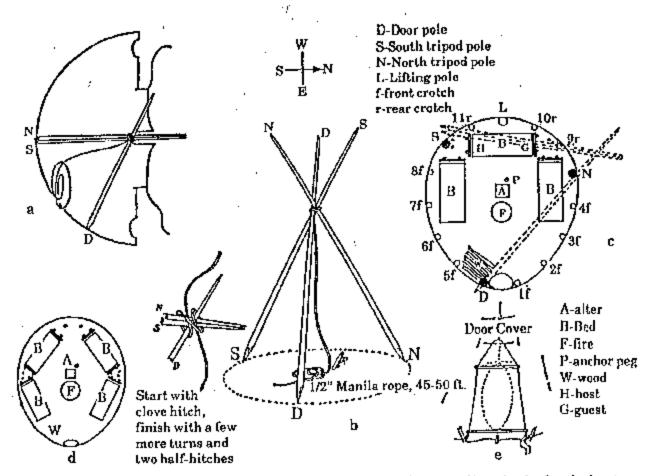
a-setting the proper tie point for tripod poles b-setup of the tripod poles c-typical set-up of interior of lodge three beds d-set-up of interior for four beds o-door cover
