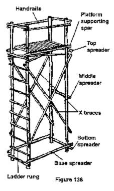
Then proceed as before. Lash on the base spreader spar and the platform supporting spar. Again, measure to make sure there's equal distance from both ends of the platform support spar to the bottoms of both legs. Continue to lash on the top long handrail and finish with the X braces.
