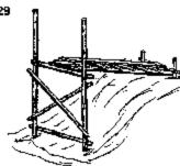
Next, put the walkways in position from both sides and lash the walkways' underspars to the transom (top ledger) of the trestle. Then drive stakes at the other end of the walkways. Lash the ends of the cross spars on the walkways to the stakes.
