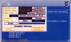
To turn this into machine code, select 'Assemble' 3 from the Program menu. A list of options will appear. Just click on Memory, and then on Assemble. Devpac will set the assembler going and ask you to press a key when it has finished.
