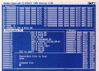
This is MonAm2, the built-in Devpac monitor. You won't need to use it for this issue. but for the curious, it's a program for taking raw machine code and turning it back into assembler. It's also rather useful for finding errors.
