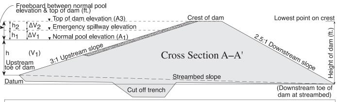
$$V_{TOD} = V_1 + \Delta V_1 + \Delta V_2$$
