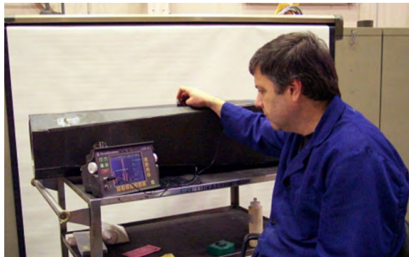
Figure 11. Ultrasonic Inspection of the Support
