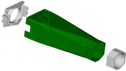
Figure 3. Tube Support Exploded View
