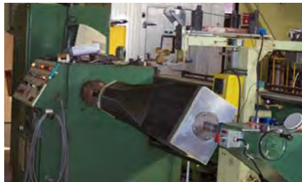
Figure 6. Filament winding the primary support shell
