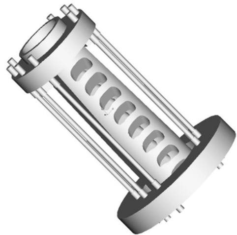
FIGURE 8. PRO/ENGINEER ® MODEL OF THE VIBRATION ABSORBER
