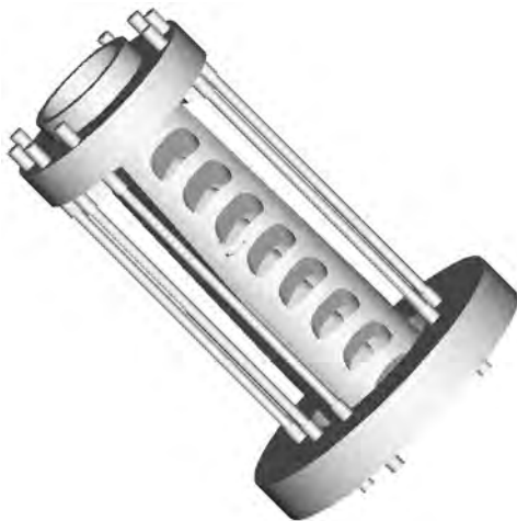
Figure 9. Pro/Engineer Model of the Vibration Absorber
