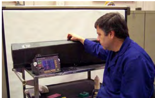
Figure 11. Ultrasonic Inspection of the Support
