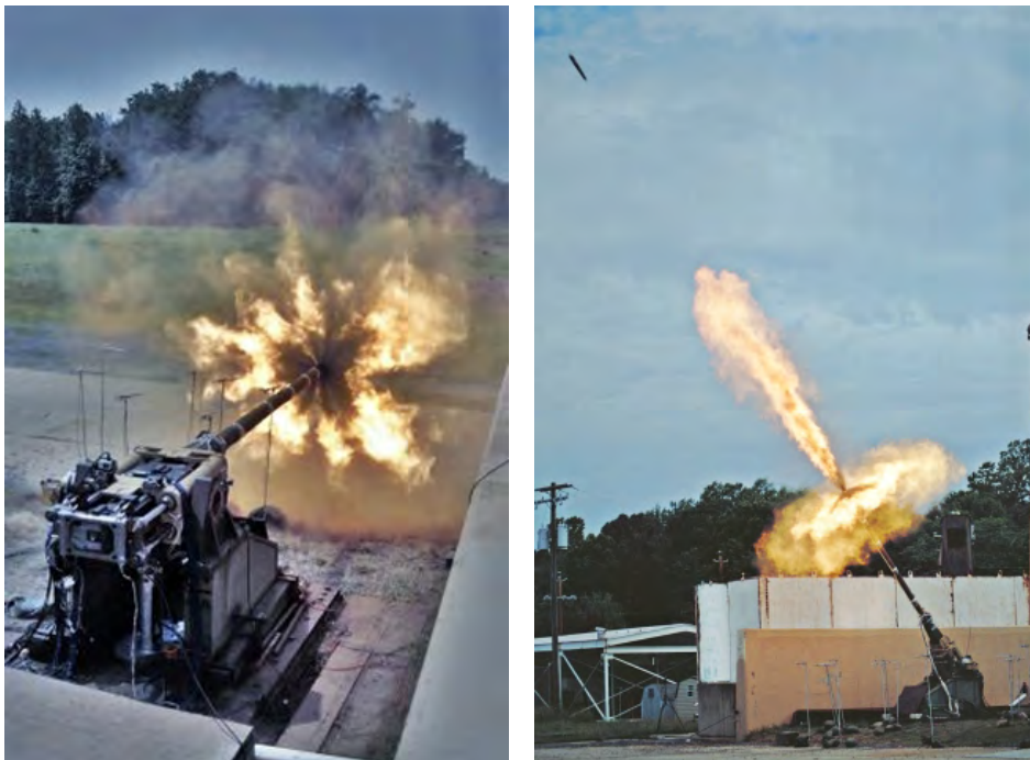
Figure 12. FCS-MRAAS Swing Chamber Launcher Direct (left) and Indirect (right) Firing
