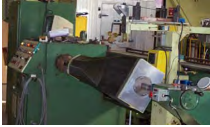
Figure 6. Filament winding the primary support shell
