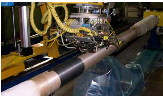
Figure 2—An axial ply being applied to the gun barrel
