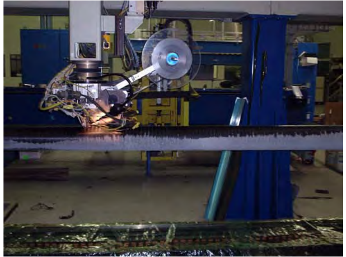
Figure 3—An Axial Ply Being Applied to the Gun Barrel
