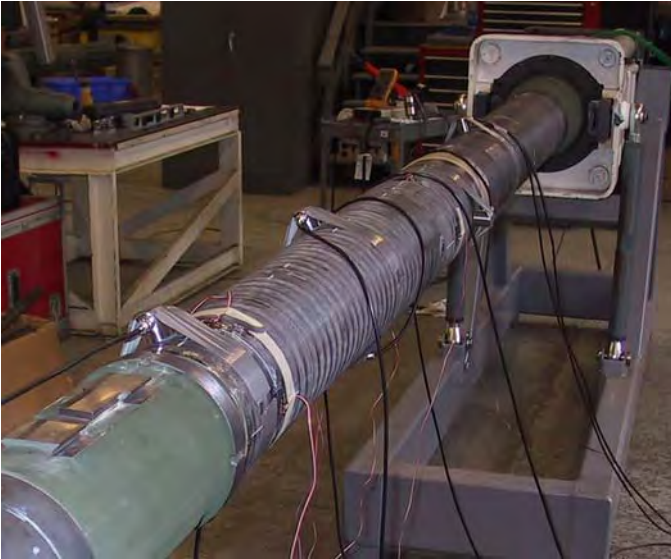
Figure 6–Acoustic Emission Test Setup
