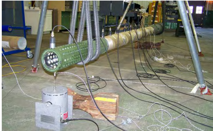
Figure 3–ATD-6 Modal Testing Setup
