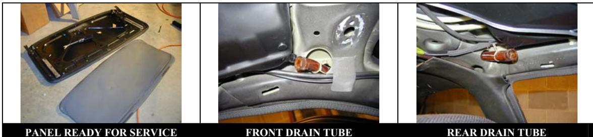
Once the sunroof panel is removed, turn on the car's ignition and actually close the sunroof assembly using the switch.
