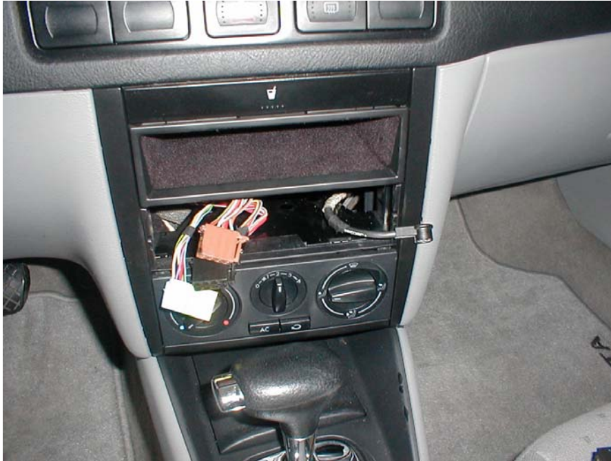
wires and antenna cable
