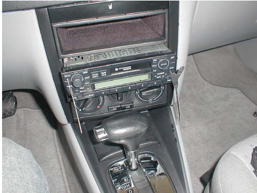
radio being pulled out with the removal keys
