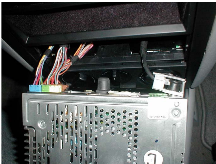
wiring and antenna connectors
