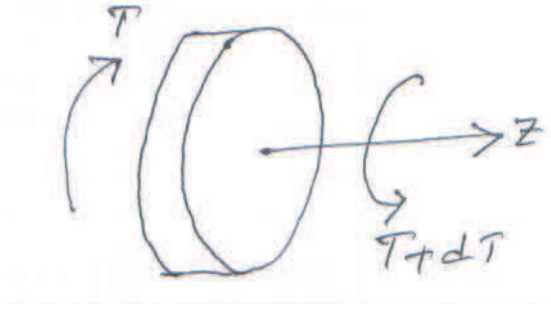
Figure 4: Angular Momentum balance of a differential element of the circular rod.
