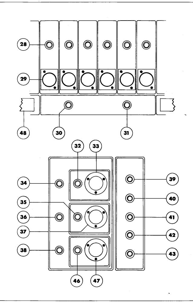
power and/or modulation. The **effects** (36) and **reverb** (38) **busses** have unbalanced outputs from their respective jacks on the rear panel. As an added feature, the 800S features a separate **stereo tape recording output jack** (34) to allow simultaneous taping during a performance when used as a sound reinforcement mixer.
