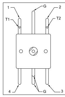
This is the pin out for the Dual 0-335pf - 0-20pf Poly Variable Capacitor. The Drawing View is looking down at the top side with the pins oriented as shown. Pins T1 and T2 are on the bottom.
