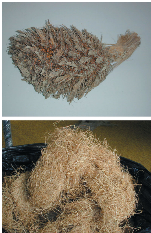
Photo. An empty fruit bunch (EFB, top) and its fibrous form (bottom).
